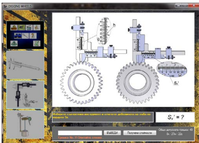
Fig.8. Measuring the chordal thickness S'_x
